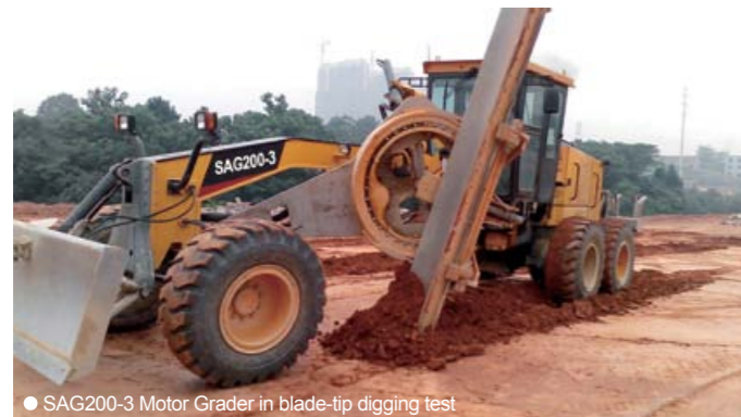
● SAG200-3 Motor Grader in blade-tip digging test
